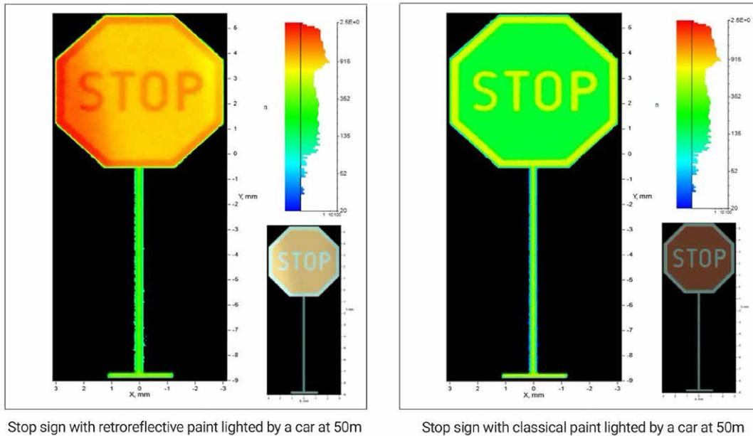
Figure 4: LightTools luminance simulations using Mini-Diff stop sign measurements
