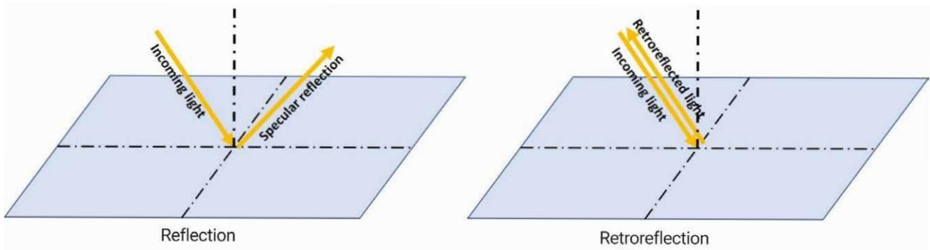
Figure 1: Illustration of reflection and retroreflection
